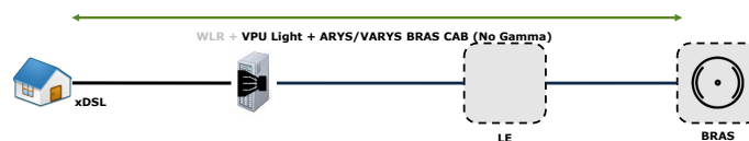
Exhibit 3.17: Illustrative representation of WLR No Gamma data transmission configuration for scenario 2
